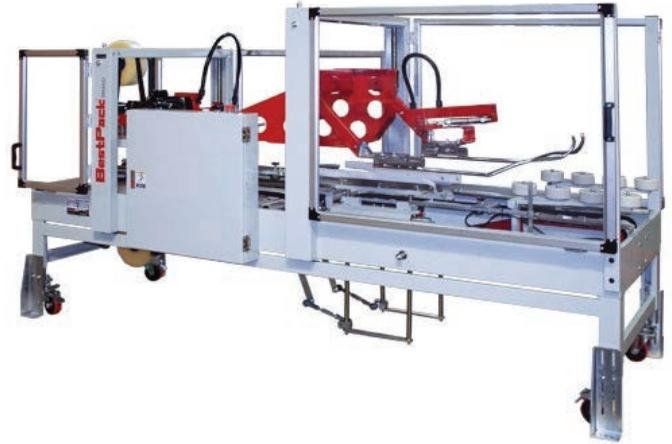
Our ATFXU line incorporates our exclusive 2" or 3" pop-out pressure-sensitive "High Speed" tape heads with BestPack's patented tab adjustment. All BestPack units are available in our standard baked enamel finish and food grade 304 stainless steel for 21 CFR 110 compliance.
