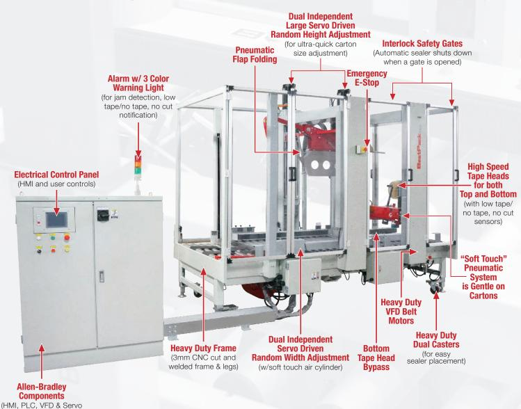
Independent Centering, Flap Folding, and Sealing Stations along with servo motor width and height adjustment allows for maximum random carton sealing speed.
