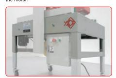
**CNC CUT AND WELDED FRAME/LEGS**
