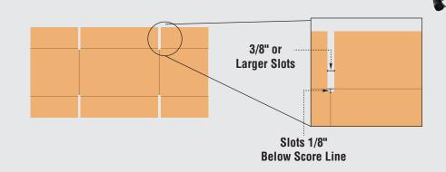
The Flap Length is to be Made Shy Cut or Scant Cut so that when the Side Panel Flaps are Folded Closed there is a 1/8" Space Between them.
