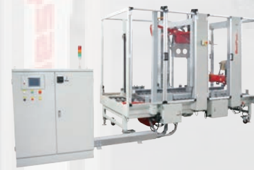
CSS Fully Automatic Servo Random Up to 30 cartons/min.
