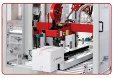
**BESTPACK'S "SOFT TOUCH" SYSTEM** Air powered belt drive and sealing section decreases product damage while maintaining presentation.
