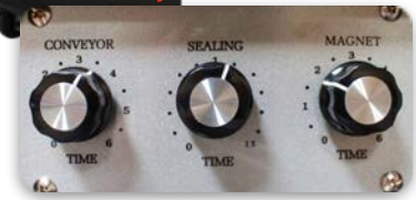
Sealer Control Panel
