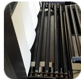
High Density Rollers - Close Roller Spacing 1/2" Gap
