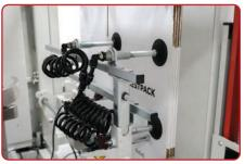
**IMPROVED PICK UP ARM DESIGN** Quickly adjust pick-up arms for carton size changes, boosting machine throughput and efficiency.
